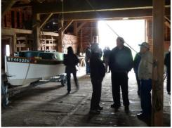
It is a 5 or 6 bay Dutch Barn- timber frame square rule barn; there are 4 regular bays and a double bay, plus an English barn added at the rear at a 90 degree angle. The original barn is about 40x60 feet, and each of the purlins is an unspliced 60 foot timber. It was built about 1820-1840. Below left, Pam & Ken.
